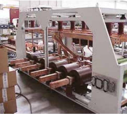
> AGN-24 Transformer for generator switchgear.
